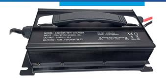
Charger for LiFePO4 (LFP) batteries with a rated voltage of 12.8V. The charging process takes place in two stages of the CC-CV, in the first stage the charger charges with DC current with a current limitation equal to the rated current of the charger. Then, when the battery reaches the appropriate voltage level, charging begins with constant voltage. The charger automatically ends the charging process.
